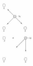
b) The upper left charge and lower right charge have equal magnitude forces at right angles to each other, resulting in a total force of twice the force of one, directed toward the lower left charge. So, all the forces sum to:
